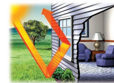
Low-E glass filters long-wave radiation from the sun. This reduces solar heat gain from the summer sun, helping to keep your home cooler.
